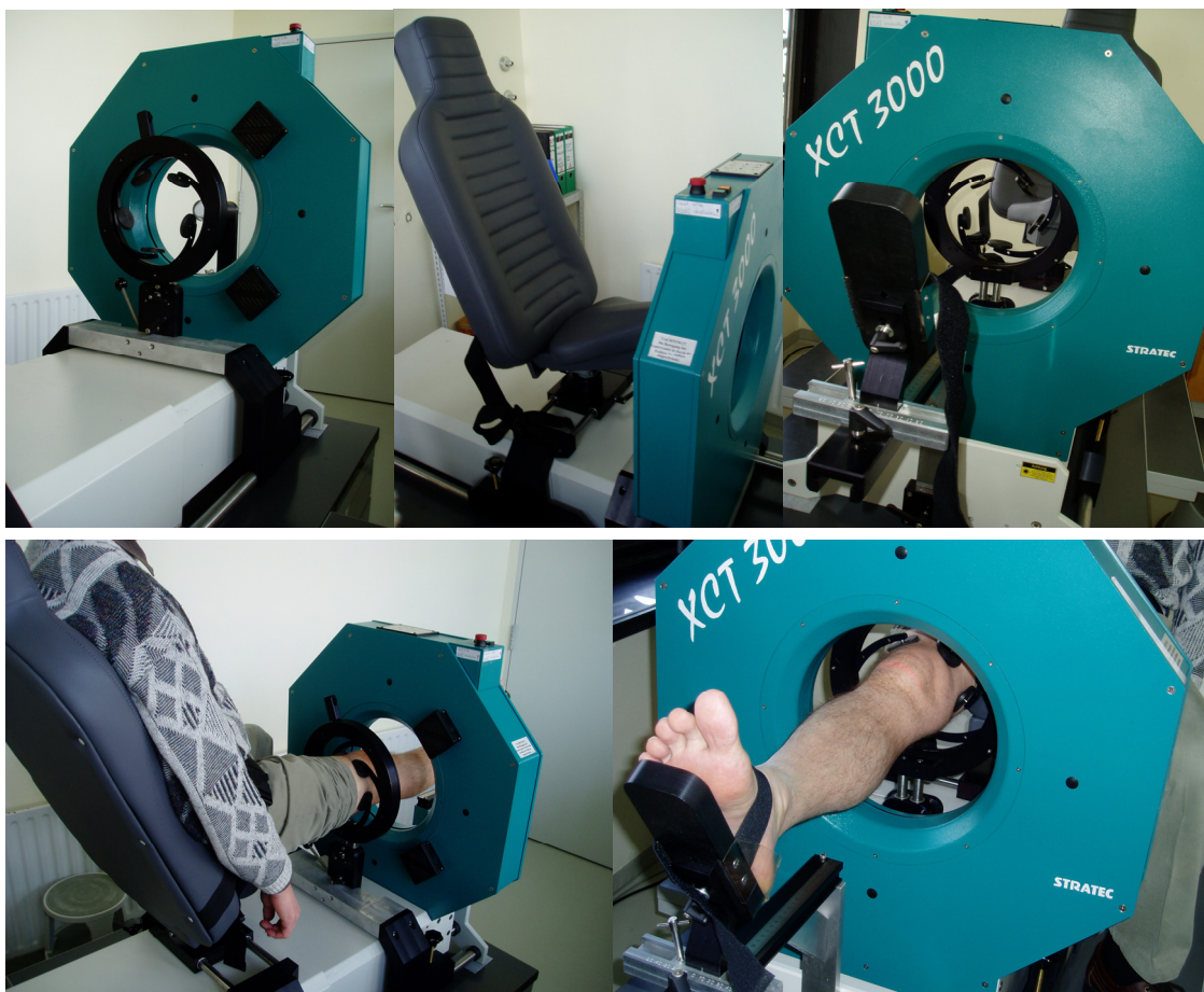
Figure 1. The pQCT-scanner allows in vivo imaging and structural analysis of proximal tibia as well as study of bone specimens from different skeletal locations.
