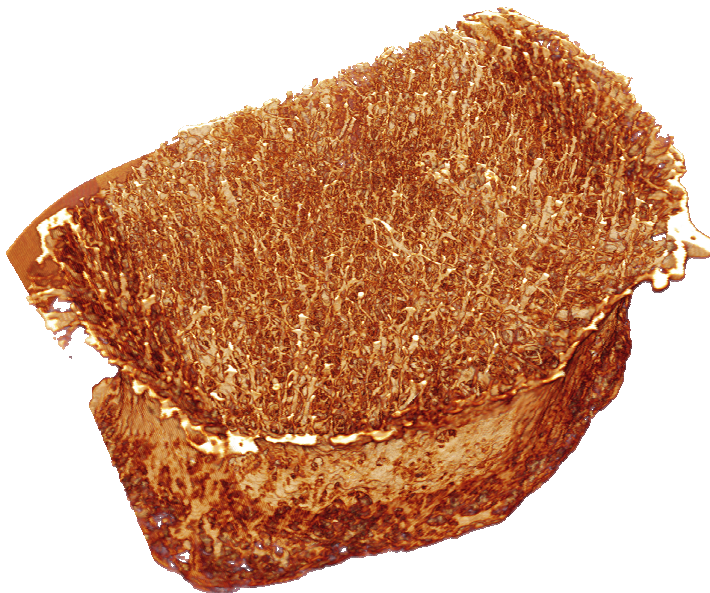
Figure 20. 3D volume rendering of an entire vertebral body and its trabecular structure (voxel size 38 \mu\text{m} ).
