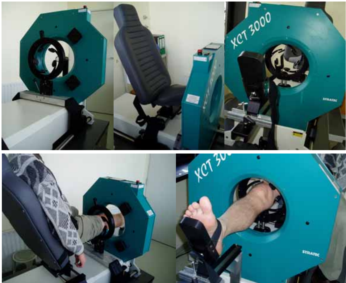
Figure 1. The pQCT-scanner allows in-vivo imaging and structural analysis of proximal tibia.
