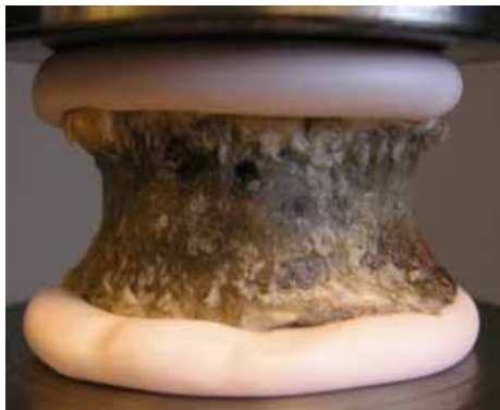
Figure 12. Vertebra L3 with interface material placed in the materials testing machine.
