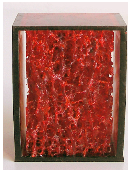
Figure 2.5. Model of trabecular bone of fourth human lumbar vertebra L4 with two additional vertical supporting walls which make the model more stable and unload bone elements during building it by RP-machine.
